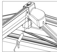
Put silicone on the gap between J23and J24, J23 and L10, J23 and the glass to prevent the rain leaking into the greenhouse.
