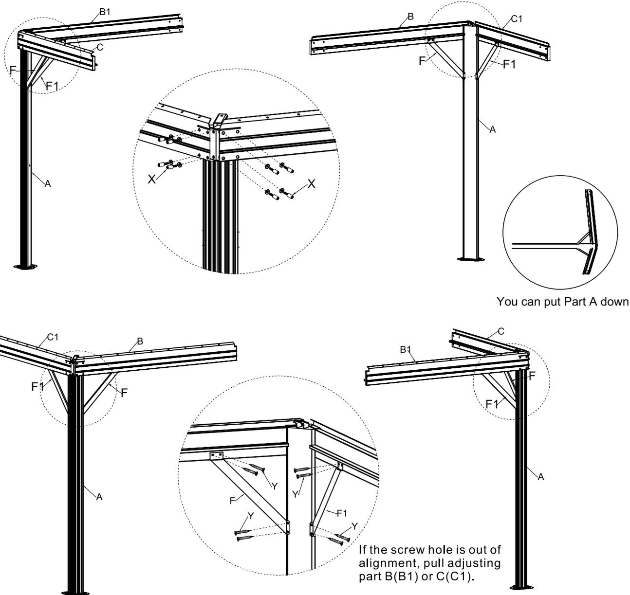
STEP 2: Attach Crossbeams 1 (Part B) and Crossbeams 4 (Part C1) to Pillars (Part A). Attach Support Brackets (Parts F and F1) to Crossbeam and Pillar. Attach Crossbeams 2 (Part B1) and Crossbeams 3 (Part C) to Pillars (Part A). Attach Support Brackets (Parts F and F1) to Cross Beam and Pillar.
