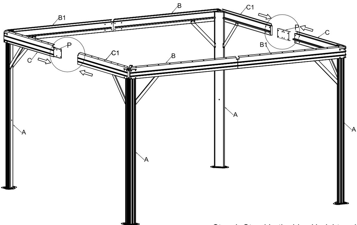
Step 4: Stand both sides Upright and Connect Crossbeams B and Crossbeams B1 using the Crossbeam Connectors (Part P).
