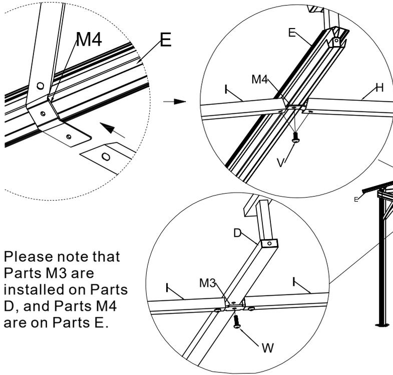
Please note that Parts M3 are installed on Parts D, and Parts M4 are on Parts E.
