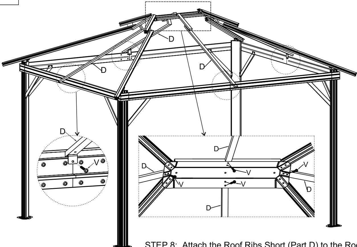
STEP 8: Attach the Roof Ribs Short (Part D) to the Roof Top Brace (Part K1). Attached the Roof Ribs Short (Part D) to the assembled frame.
