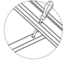
If the screw hole is out of alignment, insert it with a screwdriver and correct it
