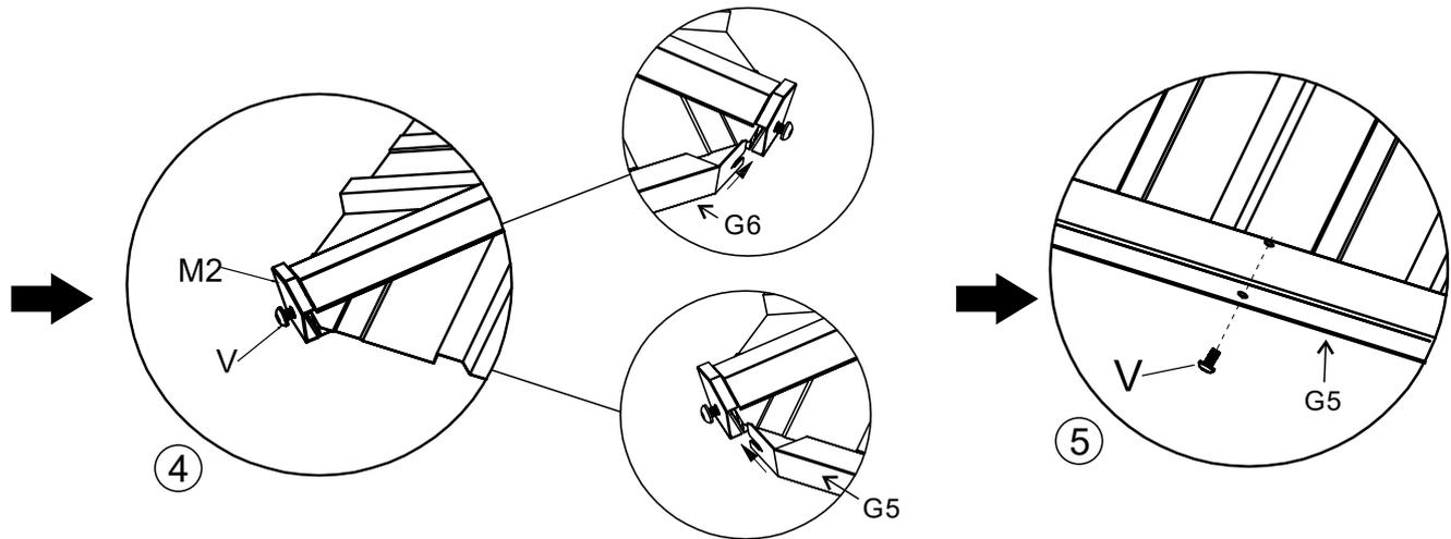
Step11-2: First fix 4 (Part M2) with V, but do not screw too tight, then install (Part G5 and G6) from left to right.
