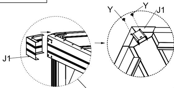
STEP 5-1: Attach the Corner Protectors (Part J1) and the Rib Supports (Part J2) Just twist the top two screws of (Part J2)
