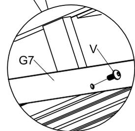
Gently insert Z2, Z3, Z4 from left to right as shown, then tighten them via screws U1 and V.
