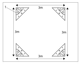
Place the four corner bases (1) at the corners of a square measuring 3x3 m.
