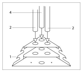
Place the longest tubes (2) in the two outermost holes in each corner base and the shorter tube (4) in the middle hole. Mount the tubes so the snap-and-click features points upwards.
