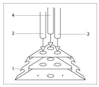
Place the longest tubes (2) in the two outermost holes in each corner base and the shorter tube (4) in the middle hole. Mount the tubes so the snap-and-click features points upwards.
