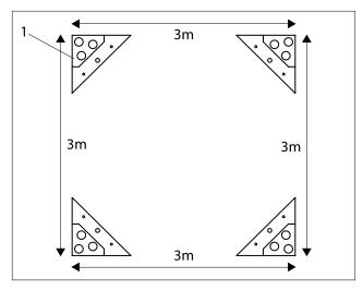
Place the four corner bases (1) at the corners of a square measuring 3x3 m.
