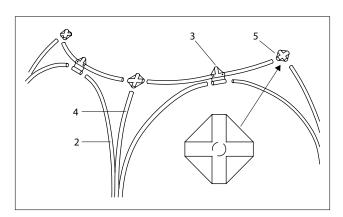
Mount the tubes (2) in (3) for a complete arch. Mount the connector (5) with the middle tube (4). Mount the horizontal tubes (3) with the connectors (5) to make a ring.
