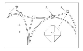
Mount the tubes (2) in (3) for a complete arch. Mount the connector (5) with the middle tube (4). Mount the horizontal tubes (3) with the connectors (5) to make a ring.
