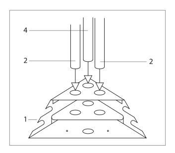
Place the longest tubes (2) in the 2 outermost holes in each corner base and the shorter tube (4) in the middle hole.
