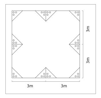
Place the 12 corner bases (1) as shown on drawing so they form a frame measuring 6x6 m. If the marquee is mounted outside use ground pegs (8) inserted into the ground with a hammer. If the marquee is mounted on a concrete or wooden floor, the corner base can be fastened with concrete nails or screws.
