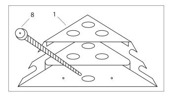
Now you can fasten the remaining corner bases if necessary.
