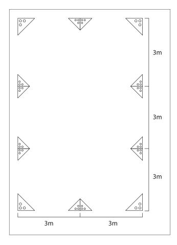
Place the 16 corner bases (1) as shown on drawing so they form a frame measuring 6x9 m.
