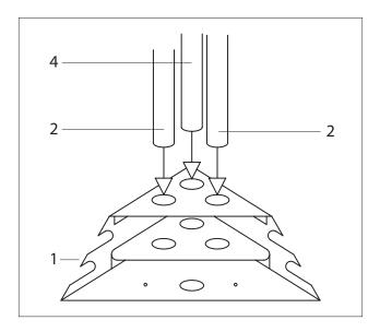
Place the longest tubes (2) in the 2 outermost holes in each corner base and the shorter tube (4) in the middle hole. Mount the tubes so the snap-and-click features points upwards.
