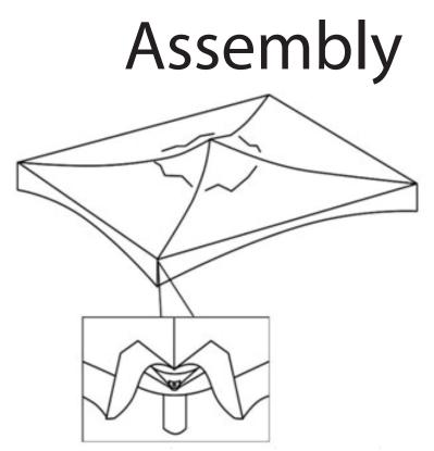
**Step 5**: Assembly the roof cover, pull the corner with handle.
