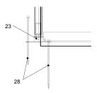
9.) Put the legs straight. Secure the tent by knitting in the anchors to the holes of the baseplate. The pagoda comes with 16 ground-anchors.
