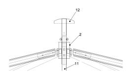
$5.)\,\text{Take}$  the mast (11) and slide it from top into the ridge-piece (2) fix the top-cap (12) over the tube.
