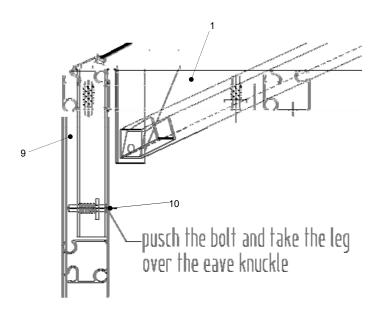
5.) Lift the 4 legs and push the bolt (10), slide the legs over the eave connector until the bolt slids in.
