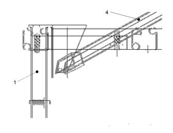
2.) Take the beams (4) and fit these in eave-connectors (1). Repeat at all four eave corners.
