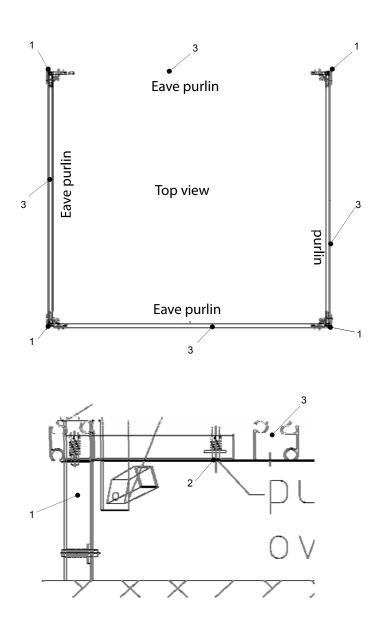
1.) Take the eave-connector and push in the bolt, then fit the eave-purlin over the tube 40x40 until the bolt (2) slids in the hole. Repeat for all 4 corners, see drawing above.
