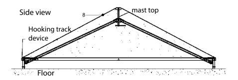
4.) Fit the top-cap (6) onto the spindle (5a) and put the roof-cover over the frame. Fix the in the channel-groove (7) of the roof-cover (8) on all 4 sides. Hook the track-device in the eave-purlins (3) and span the roof by turning the spindle (5a) until the required tensioning is reached.
