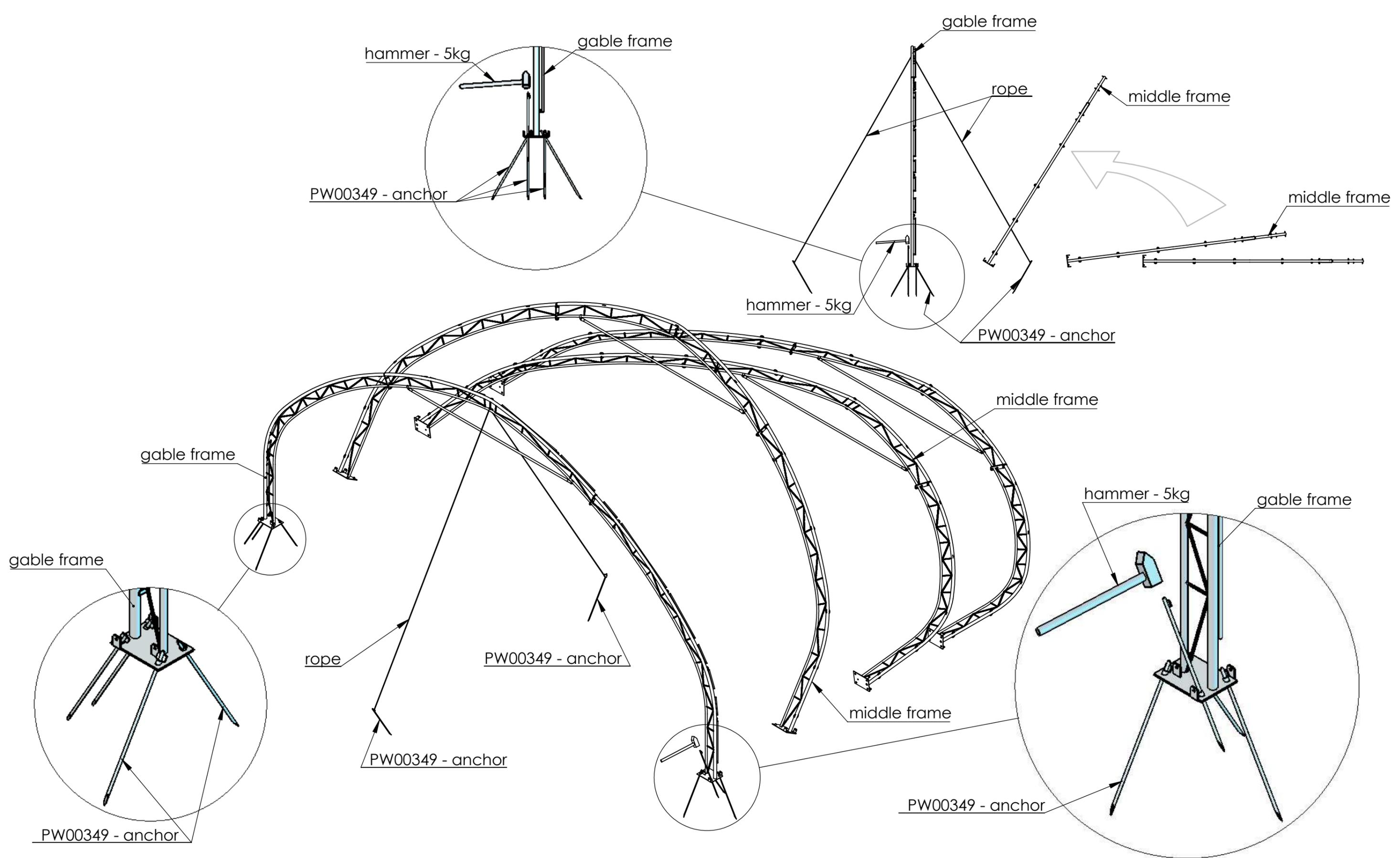
*mounting instruction - mounting of struts for first section*
