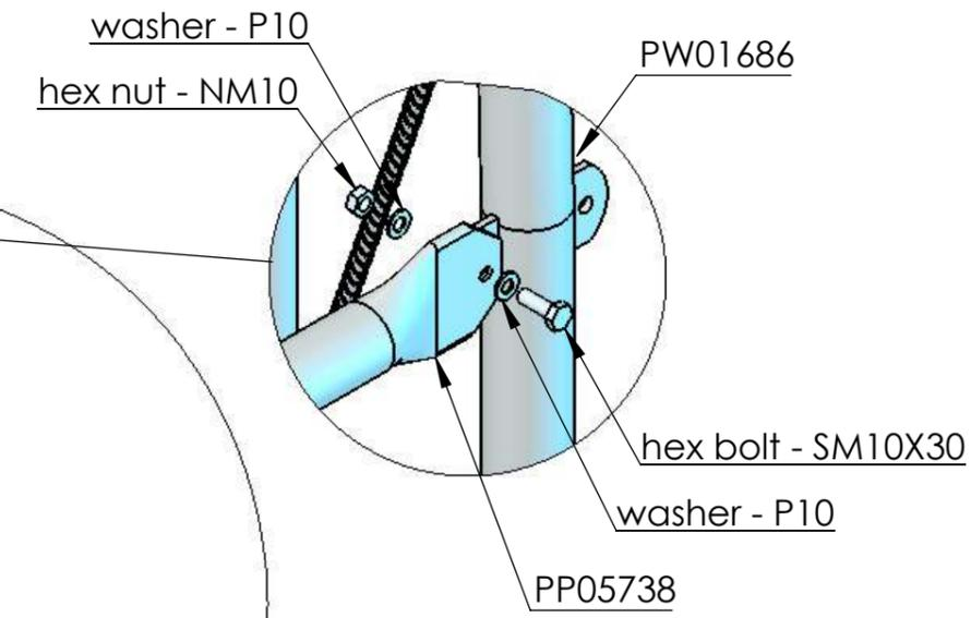
*mounting instruction - mounting of struts for first section*
