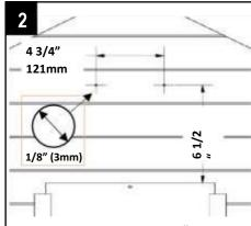
Mark two hole positions 4 ¾" (121mm) apart and approximately 6 ½" (170mm) above the top of the sliding door.
