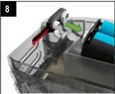
Fit the connector to the battery holder.
