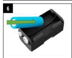
Fit the batteries into the holder.
